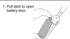
Insert 2 AA batteries according to correct polarity marked inside battery compartment. Reattach battery door when finished.
