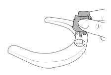
Slide magnifier handle into adapter. Magnifier is keyed to fit one way. There will be an audible click when handle is inserted correctly.
